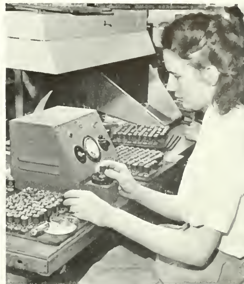
BEFORE THE ELEMENTS ARE SEALED INSIDE THE TUBE, EACH PART IS CAREFULLY TESTED FOR PERFECTION.
